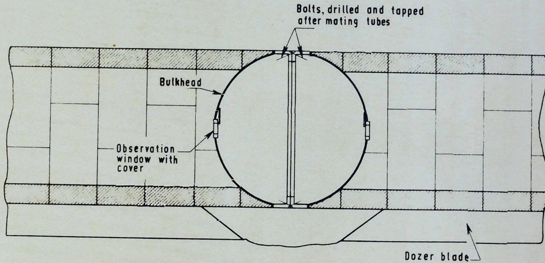
Fig. 4 Arrangements for joining tubes at mid-channel
